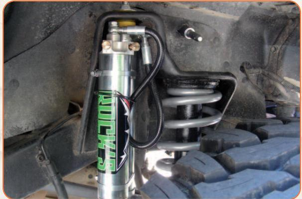
*Rock's Extreme Duty mono-tube gas shock with compression adjustment specific for TJ. The larger gas chamber allows for far greater tolerance to the oil expansion and pressure increase that occurs as operating temperatures climb inside the shock. Completely serviceable.*
