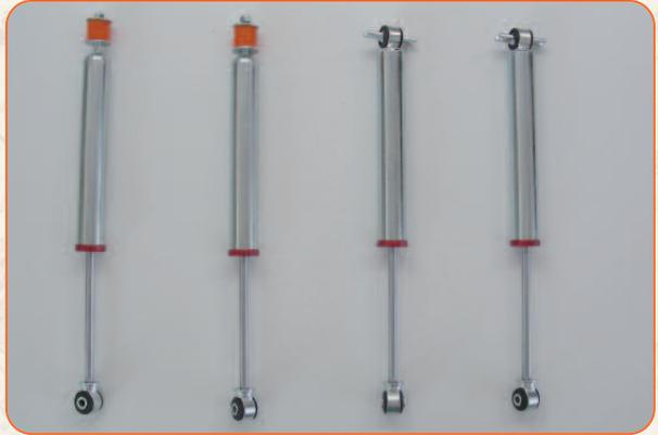
*Rock's mono-tube gas shock specific for TJ are developed and tuned specifically for each application to deliver maximum control while not compromising ride quality, high speed stability and comfort for those extended trips over the toughest terrain. Completely serviceable.*
