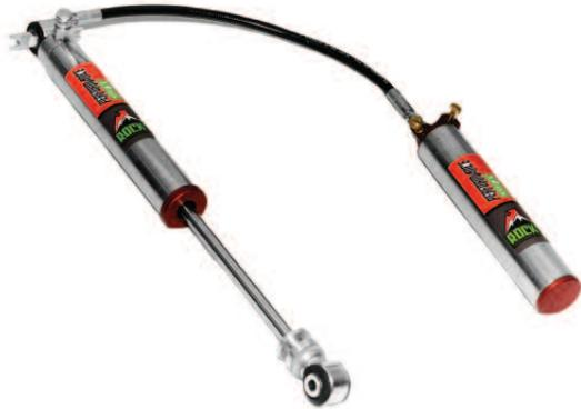
*Rock's Extreme Duty mono-tube gas shock with compression adjustment specific for JK. The larger gas chamber allows for far greater tolerance to the oil expansion and pressure increase that occurs as operating temperatures climb inside the shock. Completely serviceable.*
